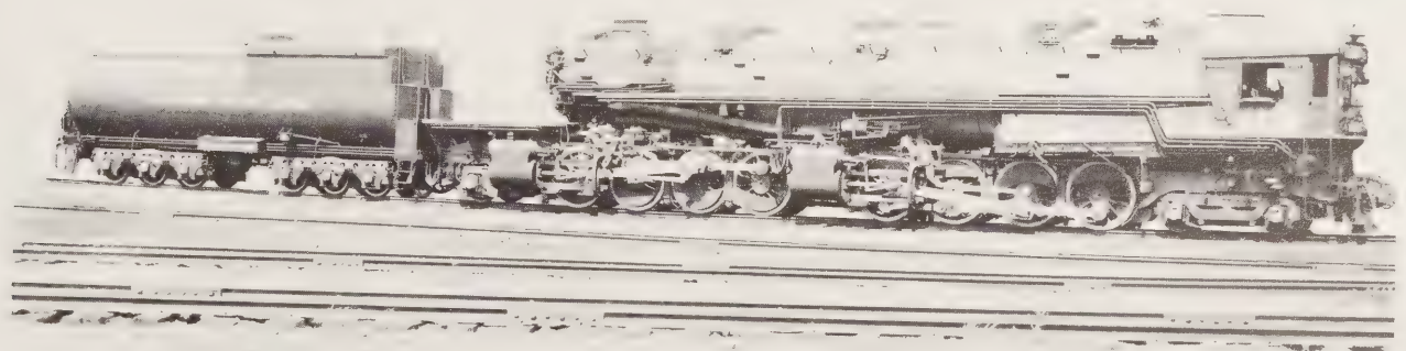
One of the Single Expansion 4-8-8-2 Type Locomotives, Built by The Baldwin Locomotive Works in 1930
